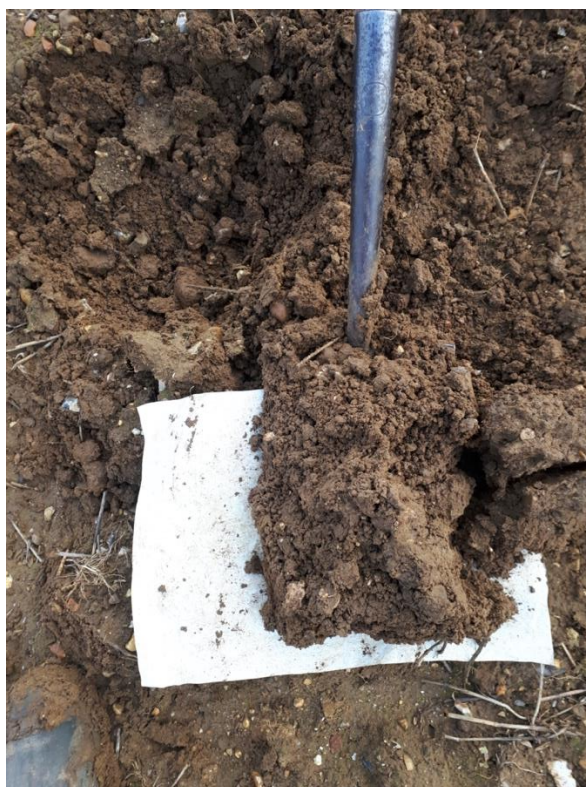
Figure 2 Visual Evaluation of Soil Structure, farmer-photographed block. Medium texture, cropping-rotation including late-harvested crops. Most limiting layer score 3. Accompanying notes describe a crumbly structure for 10-15cm over larger angular blocks.
